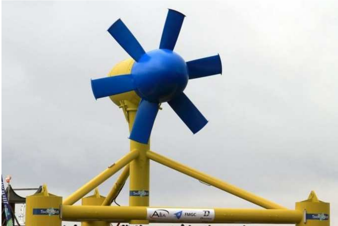
Figure 28: Sabella D10 turbine before offshore installation
