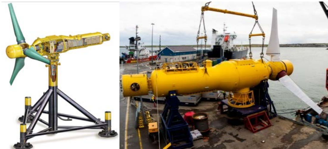
Figure 1: DEEP-Gen IV tidal turbine; modelled on the tripod (left) and prior to the first deployment (right)
