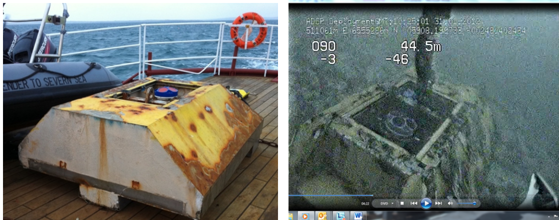
(a) Pre-deployment. UoE ADCP in TGL seabed frame. Image c/o Liam Warren TGL Ltd.
