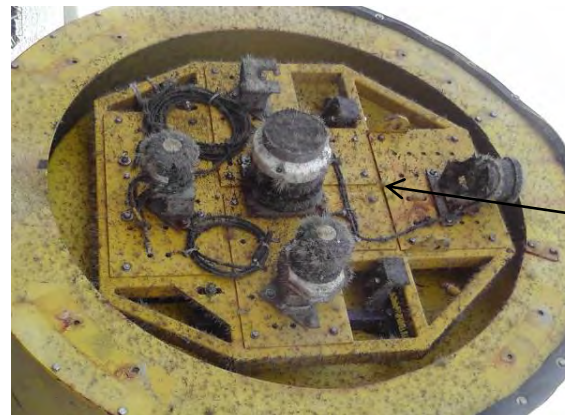
Fouling on the thruster
