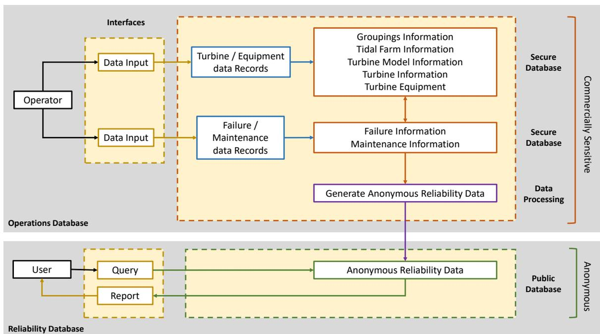
Figure 8-1 - Schematic of reliability database data flow.
