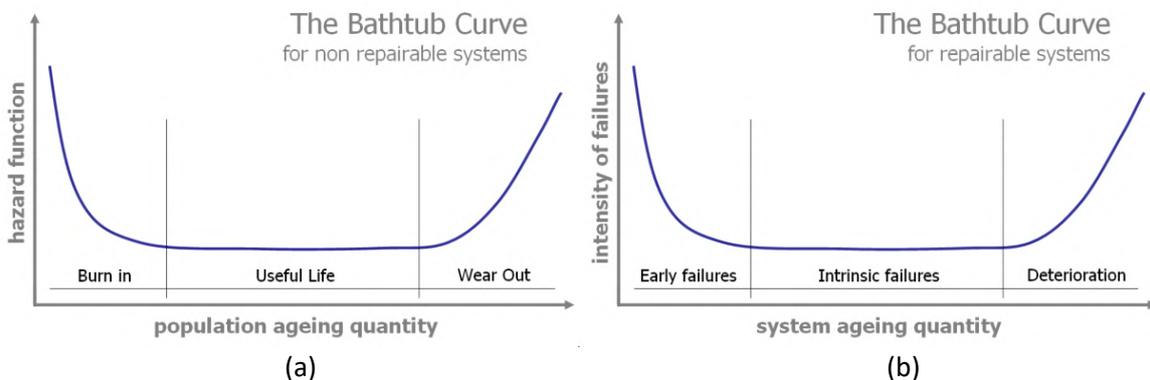
Figure 4-2 - The bathtub curve (a) for non-repairable systems and (b) for repairable systems [26].
