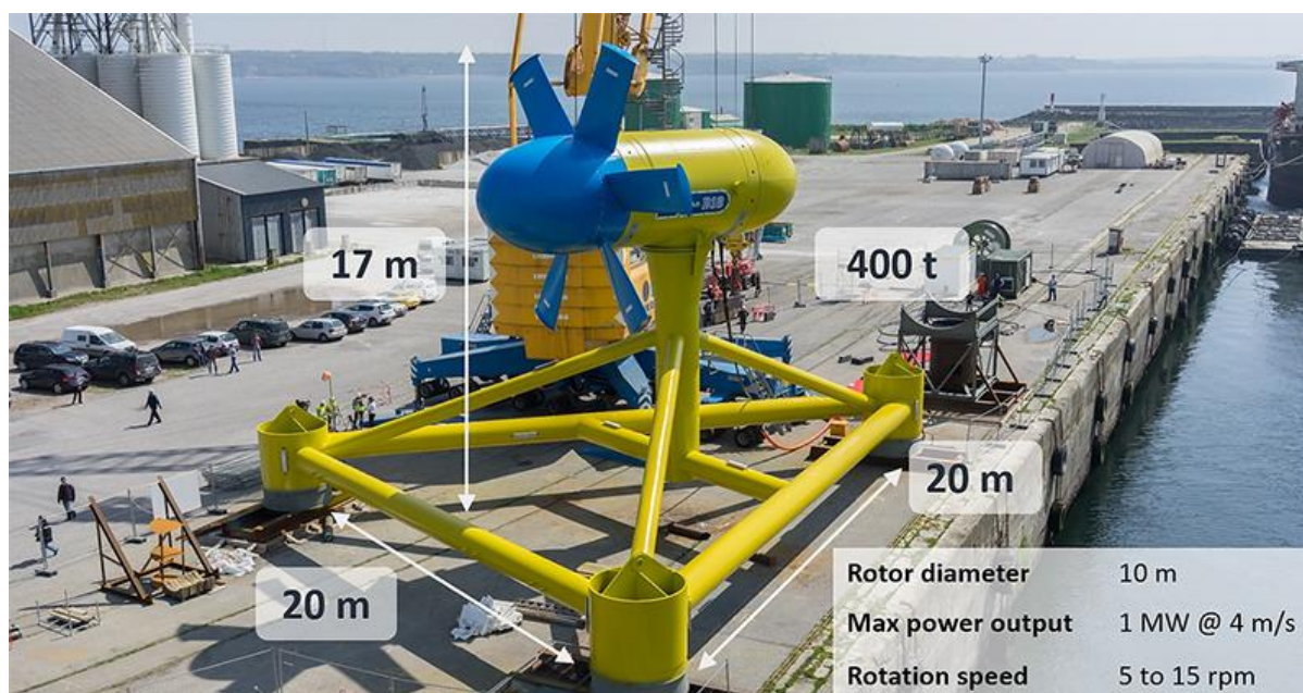
Figure 4. Sabella D10 turbine dock arrangement. Source: Sabella website
