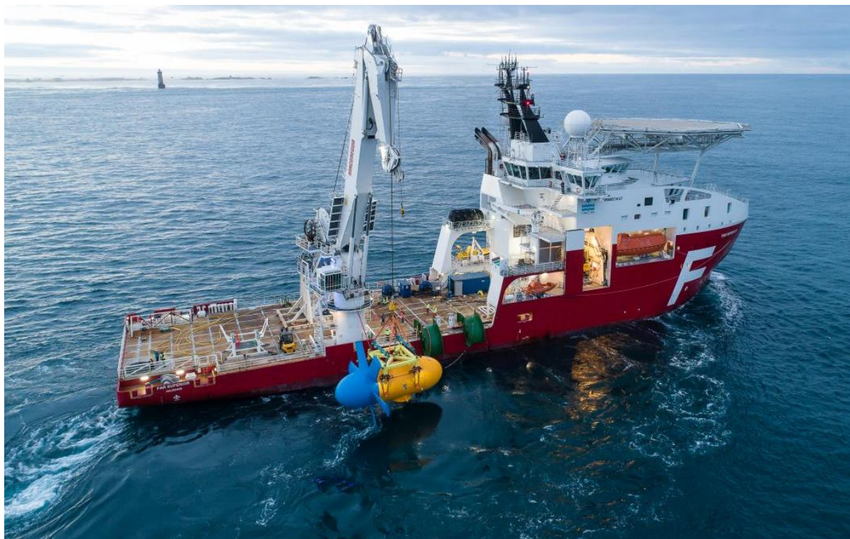
Figure 5. Installation of the Sabella D10 turbine. Source: Sabella website
