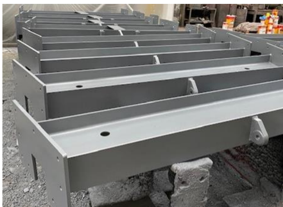
Frame sections awaiting final top-coat of marine paint
