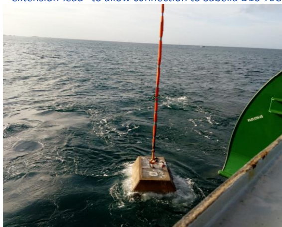
RealTide ADCP being lowered to ~58m depth in Fromveur Strait September 2019.
