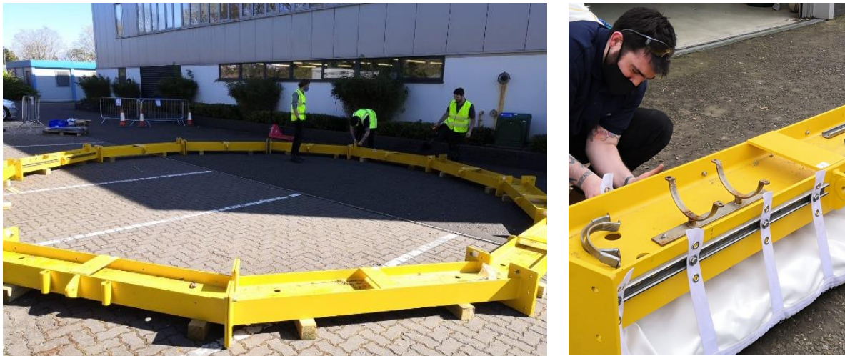
Figure 3-22. Frame assembly tests at FloWave (left). Test fitting additional compliant ballast bags (right).
