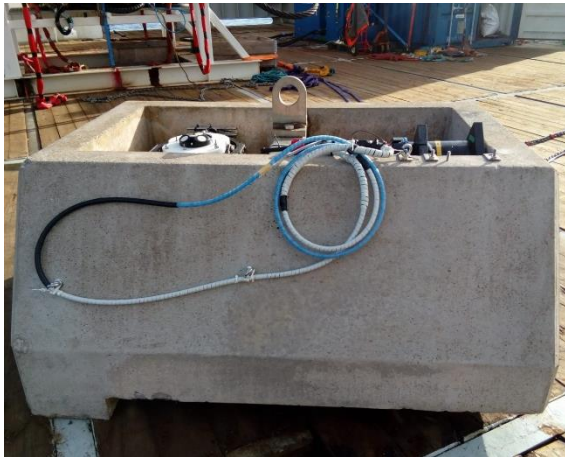
UEDIN concrete gravity mooring with diver connectable "extension-lead" to allow connection to Sabella D10 TEC
