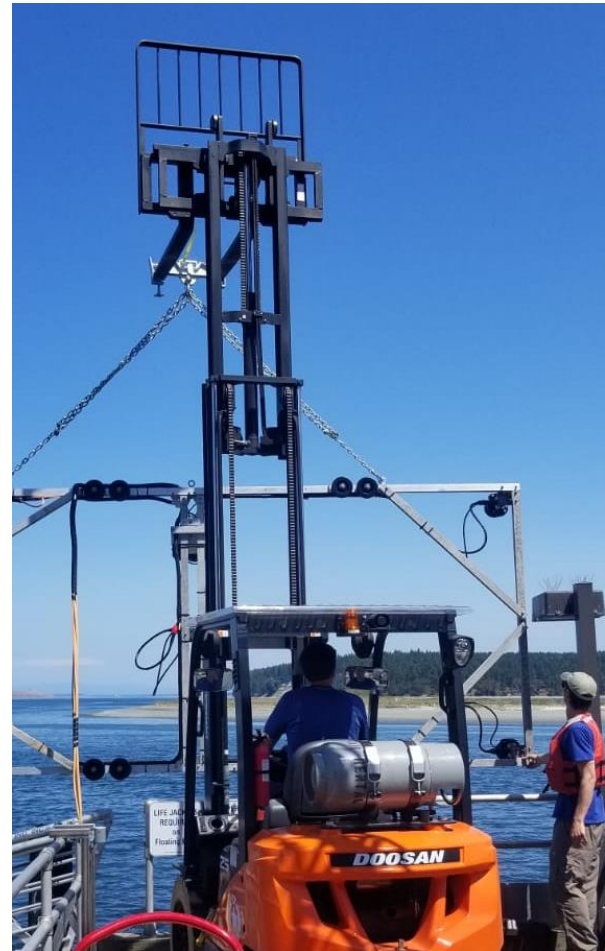
Figure 3-16: Implementation: laboratory testing at PNNL, USA showing system verification tests underway. Torches have been affixed aligned to the S-BD profilers and the system is undergoing actuation tests to verify coordinate transforms (Note: the white lines are overlaid for clarity) (left) and (right) field installation via forklift off the pier at the Marine and Coastal Research Laboratory, PNNL, Sequim, WA, USA.
