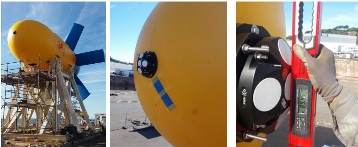
Figure 3-5: Sabella D10 turbine rear bulb showing Nortek Signature 500 installed in horizontal orientation to capture behind-turbine (on ebb tide) and ambient-to-turbine inflows (on flood tide) at turbine hub-height.
