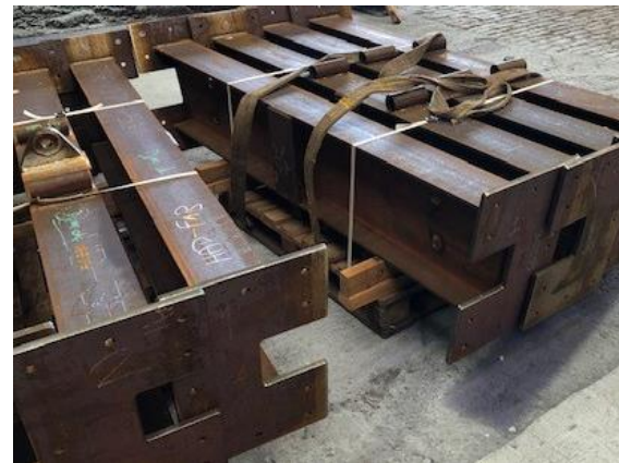
Frame sections post-fabrication awaiting cleaning and coating
