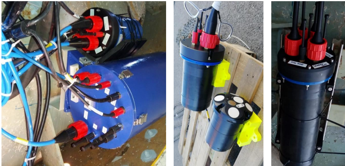
Figure 3-3: Iterative development of instrument control boxes (ICBs) from left to right featuring altered internal components (smaller with more redundancy) to affect increased resilience.
