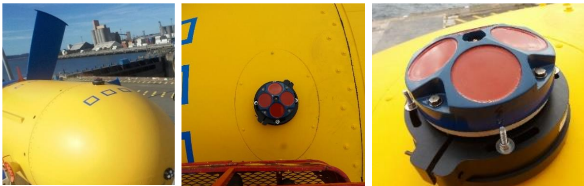
Figure 3-4: Sabella D10 turbine rear bulb showing RDI Workhorse Sentinel 600 installed in vertical orientation to capture above-turbine current flows and wave action.
