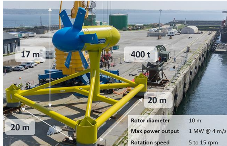
Figure 2 – Tidal turbine tested at FloWave (left) and Sabella D10 before deployment (right) [2].
