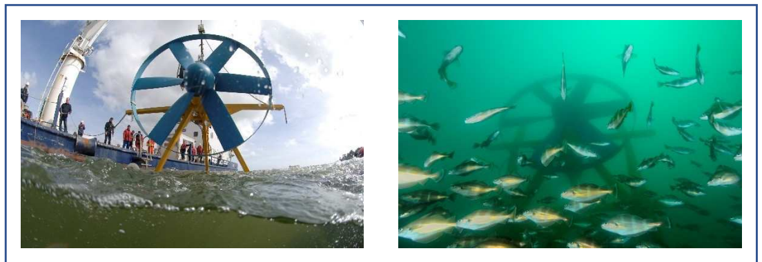
Figure 5-5 – Sabella D03 tidal turbine trial
