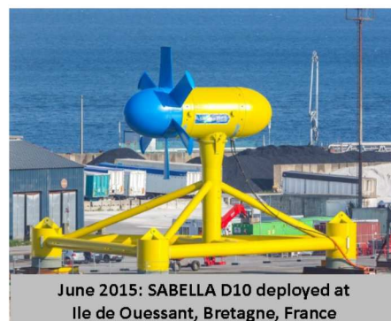
Figure 5-6 – Sabella D10 scale prototype and full scale comparison
