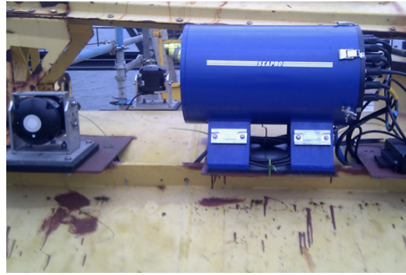
(a) Installing instrumentation to the 500kW turbine on site at Hatston Quay, Orkney (b) Instrumentation and instrumentation control-box installed on the 500kW machine
