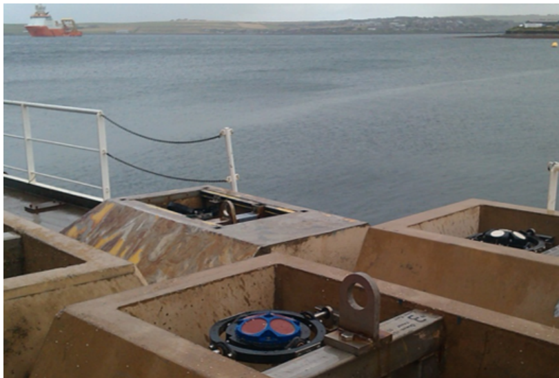
(a) Type B (top centre) and Type C (others) ADP frames with RDI Workhorse Sentinel ADCP installed (bottom centre) and Nortek Signature 500 installed (right). Positioned on a crane barge at Hatson Quay, Kirkwall prior to uplift by the deployment vessel.
