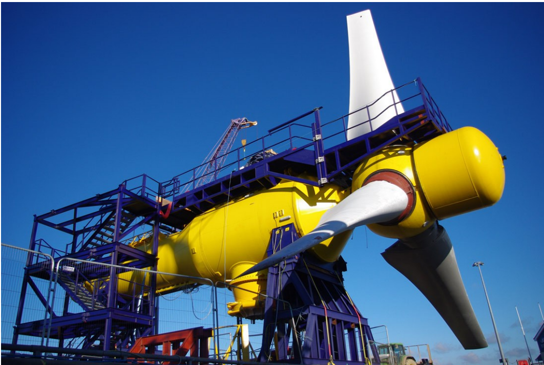
(b) The 1MW DEEPGEN IV on stand.
