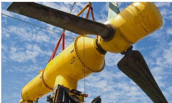
(a) The 500kW DEEPGEN III being lifted.
