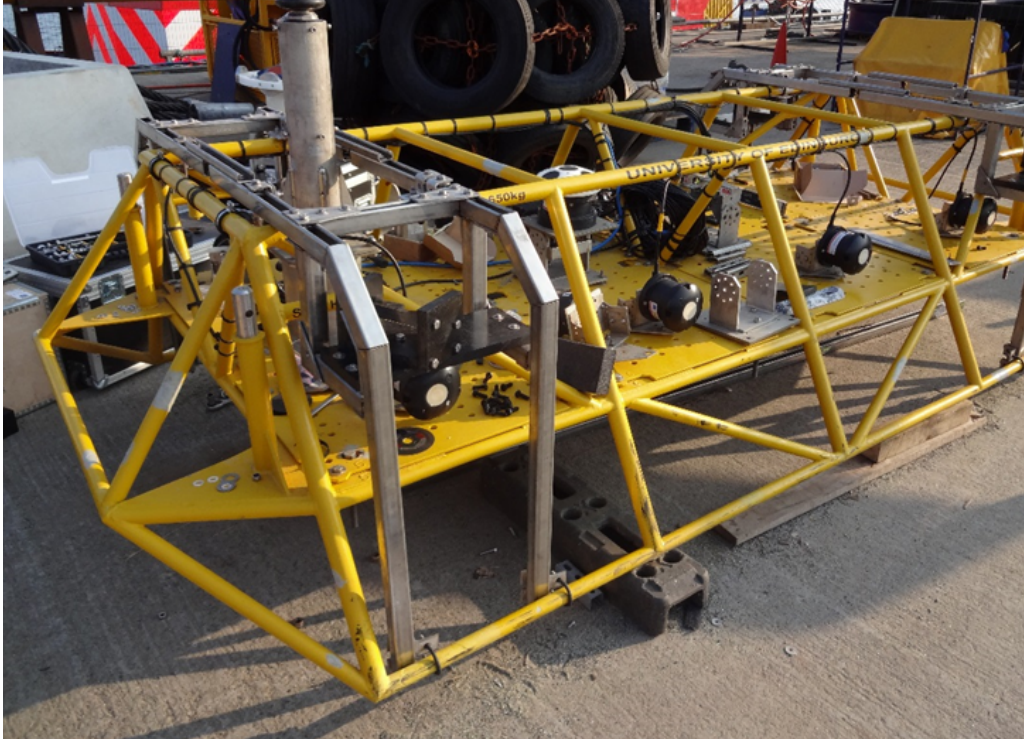
(a) Photograph of ESIP-1 taken summer 2014 prior to deployment. Undergoing repair and maintenance and recently upgraded to allow mounting of C-ADP corner instruments.
