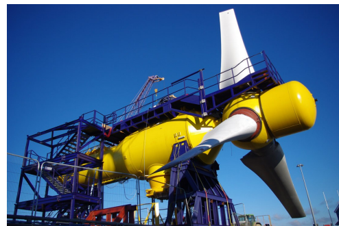
(b) The 1MW DEEPGEN IV on stand.
