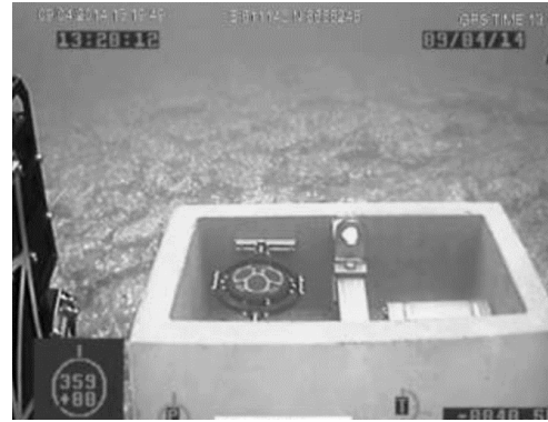
(b) Recovery of ADCP from seabed using ROV
