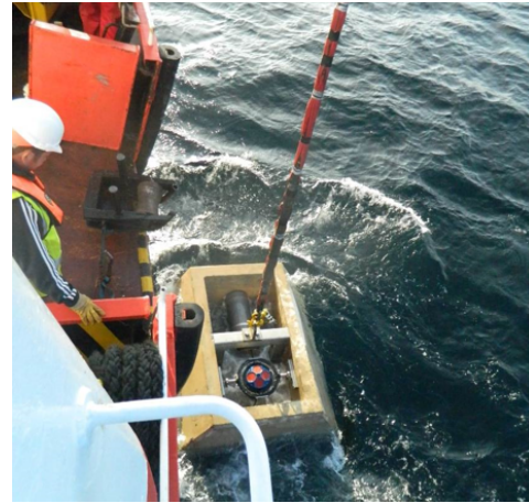
(b) RDI ADCP in Type B ADP frame being deployed
